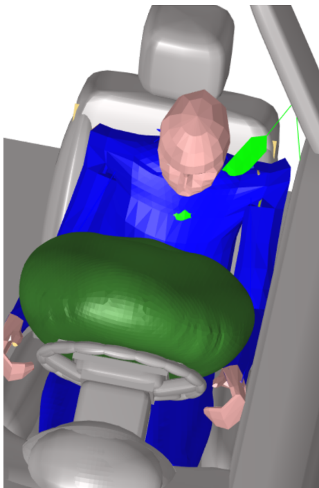
(a) Active human body model of an occupant placed inside a generic vehicle interior.
